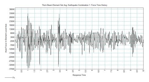
Peak results for the averaged element forces and moments are displayed in Notepad in file **peak\_forceSet\_Avg1.sum**. These indicate a peak positive average axial (Fx) force of 32.7kN at solution time 0.98 seconds and a peak negative average axial (Fx) force of -36.1kN at 1.01 seconds for the 1940 El Centro earthquake (Record 1), as shown in the following figure.
