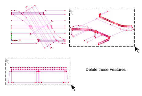
The DXF features are imported in scaled units defined by the drawing scale. These features will need to be scaled to suit the units of the analysis. Only the features defining the plan view are to be used in creating the analysis model. All other features can be deleted.
