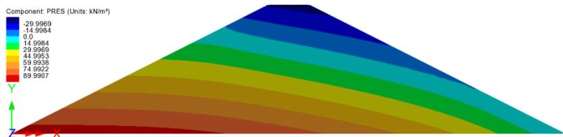
Figure 10: Pore pressure contour (water level at 10 m)
