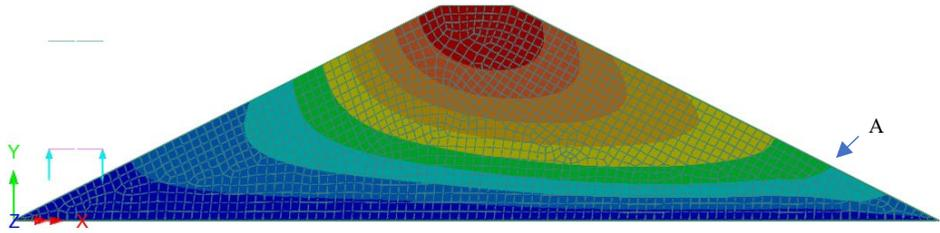
Figure 11: Resultant displacement (water level at 10 m)
