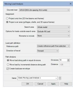
Loadcases 3 to 13 that represent the HB load moving forward across the bridge will be generated in the Treeview along with a maximum and minimum load envelope.
