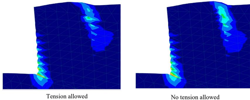
**Figure 10: Effective strain after installing final nail**
