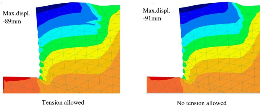
Figure 9: Horizontal displacements after installing final nail
