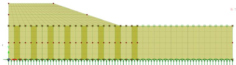
Figure 9: Boundary conditions at embankment construction stage
