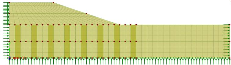
Figure 7: Boundary conditions at initial stage
