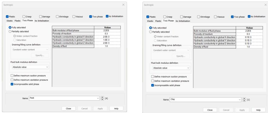
Figure 5: Two-phase properties for clay and peat layers
