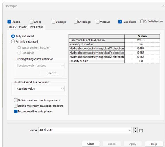
Figure 6: Two-phase properties for sand drains
