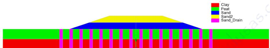
Figure 1: Embankment model
