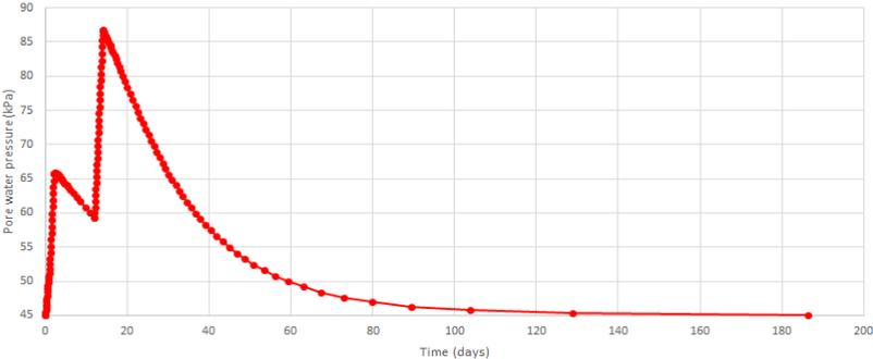
Figure 22: Variation of pore pressure with time
