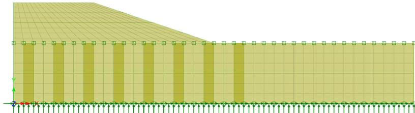
Figure 16: Second layer of embankment stage (analysis 2)
