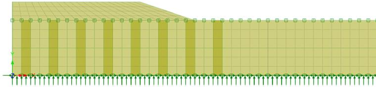
Figure 13: First layer of embankment stage (analysis 2)
