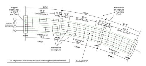
Four girders form each span, with support and intermediate bracing between them as shown on the image above. Lateral restraint is provided to the two internal girders at each support. Longitudinal restraint is provided to all four girders at pier 3. Transverse girder spacing and slab cantilever dimensions are shown on the following image, which also shows the modelling methodology used.
