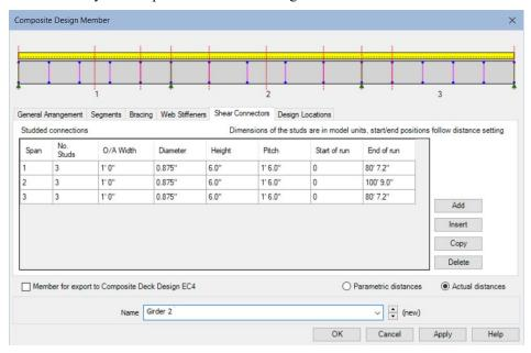
Shear connectors are represented on the schematic design member by dotted horizontal purple lines within the slab showing the length over which they apply.
