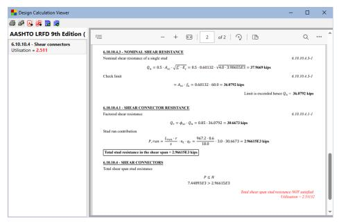
A larger stud and/or a closer pitch locally by the failure zone (by the internal supports) will be defined to try and obtain the required capacity.
