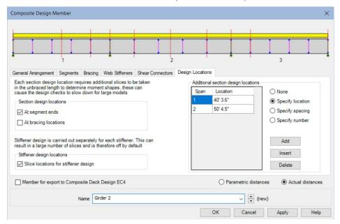
Design locations for segment ends and bracing locations are represented on the schematic design member by vertical red dotted lines. Bracing locations are shown by blue circles. Stiffener locations are shown by magenta lines.
