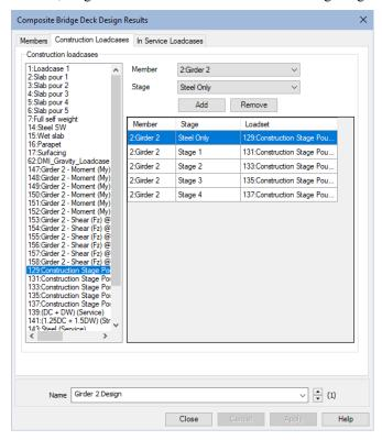
Note, again, that there is no need to add Stage 5 because design checks in the construction stage are only carried out at locations where the slab is not present.
