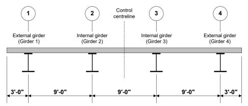
Girder and slab thickness are as follows:
