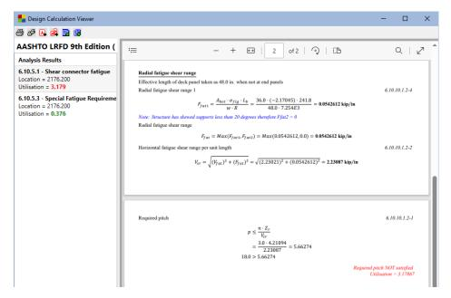
It can be seen that the required pitch of stiffeners is not satisfied. The use of a larger stud and/or a closer pitch locally by the failure zone (by the internal supports) would give the required capacity. This is covered at the end of the example.
