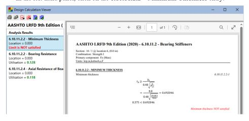
It can be seen that, for both stiffener types, the Minimum Thickness check is not satisfied. This can be resolved by increasing the thickness of the stiffeners. This is covered at the end of the example.
