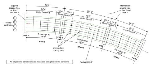
The bridge consists of three spans of length 80 feet, 100 feet and 80 feet. The bridge follows a radius of 600 feet along the control centreline and all supports are along radials. There are four girders across the width of the deck with stiffeners and bracing provided at supports and fifth point intervals along the span lengths. The deck cross-section is shown below. This example considers the design of one of these girders – Girder 2 along with the design of stiffeners.
