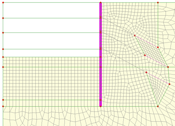
Figure 25: Excavation of fourth layer
