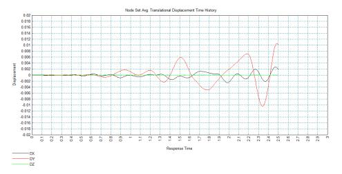
The peak results for the averaged node displacements are displayed in the Notepad file **peak\_dspSet\_Avg1.sum**. These indicate absolute peak average displacements of 0.0027m at time 2.4725 seconds in the X-direction and 0.0106m at time 2.485 seconds in the Y-direction.
