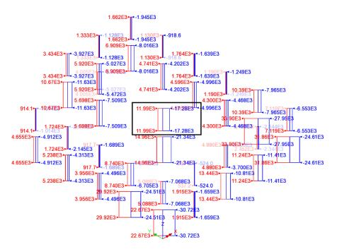
• In the Treeview right-click on the Whole Earthquake (Max) envelope and select the Set Active option to set this envelope active. Select entity Force/Moment of component My. Ensure that Change existing drawing layers to above component is selected, then click the OK button.
