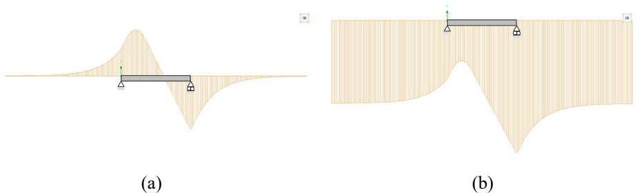
Figure 6: Rail Stresses due to Temperature Variations for a Simply Supported Deck (a) Temperature Increase in the Deck Alone, (b) Temperature Increase in the Deck and Rail
