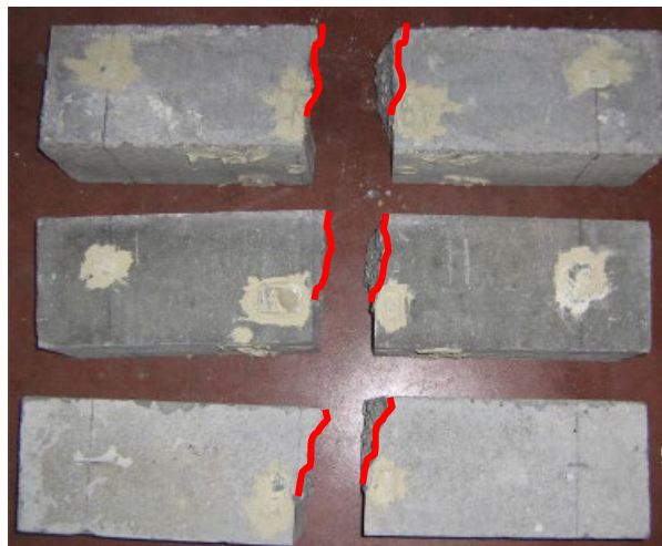
Figure 5: Failed specimens (PC) show a localised crack propagated from the notch to the top face mostly following a vertical path. Figure reported in Bencardino et al [1] has been modified to highlight matching cracking faces from each half of the beams.
