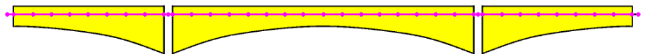
'Flat' modelling method (where lines follow the centroid of one section with other sections offset to align to match)
