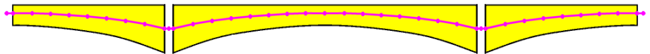
Indicative diagram showing 'Curved' modelling method (where all lines follow the centroid of sections)
